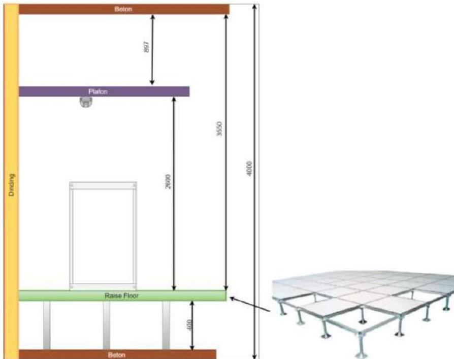
Gambar 40. Layout *Raised Access Floor*
